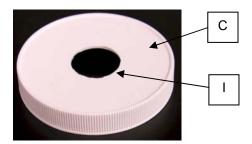
C. Lid, plastic, with screw threads to fit the standard liter (quart) size jar (Figure 1, Item D), with drilled center hole
