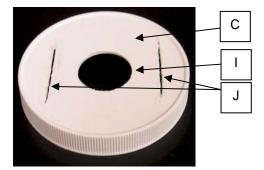
C. Lid, plastic, with screw threads to fit the standard liter (quart) size jar (Figure 1, Item D), with drilled center hole
